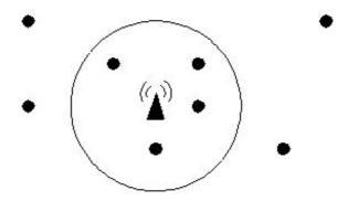
The picture above shows eight points of interest (little circles) and one of the possible optimal BTS positions (small triangle). For the given distance R, it is not possible to cover more than four points. Notice that the BTS does not need to be placed in an existing point of interest.
